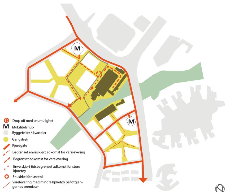
Figur 12: Diagram vareleveringsprinsipp. III. LPO/BK
