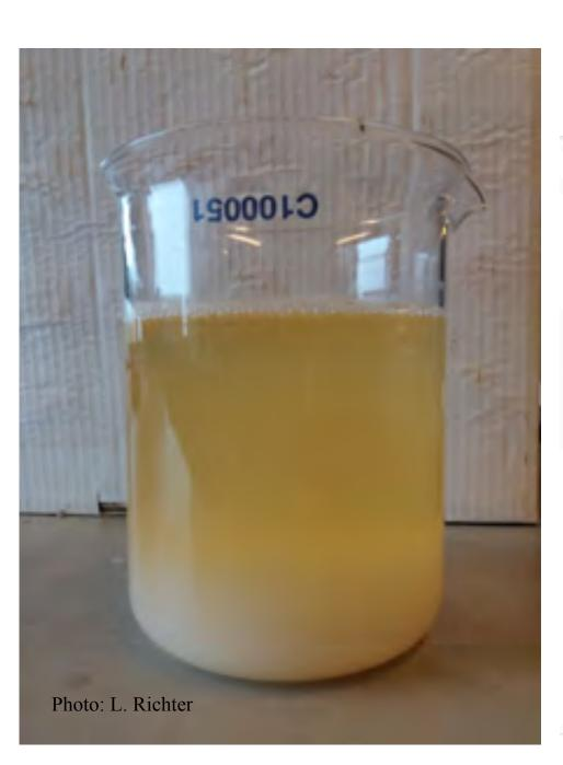
Precipitation of STRUVITE with MgCl and seawater
