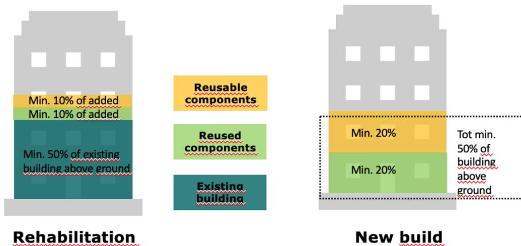
The figure illustrates quantitative criteria for reuse and reusability for circular buildings (see sections 2.3 and 2.4).
