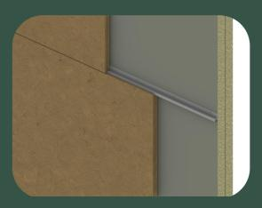
2x 40 mm Ecopanely are screwed together without studs, and 22 mm Lemix mounted onto it without screws.
